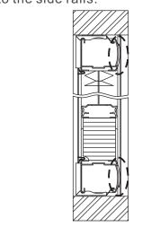
Lock the head rail brackets into the top side of the window frame.
