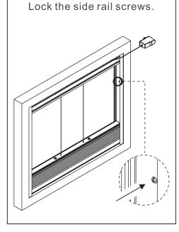
Lock the other side rail screws (locking tightly).
