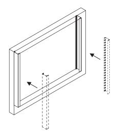
Install the head rail brackets to be positioned to let the front side of window shade can be affixed to the side rails.
