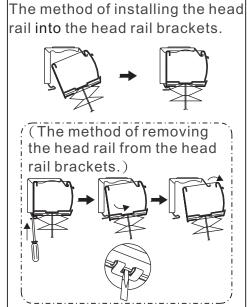
Press the down button on the remote control, install the head rail into the head rail brackets at the top.
