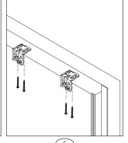
Lock the head rail brackets into the bottom side of the window frame.
