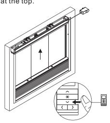
The method of installing bottom rail into the head rail brackets.
