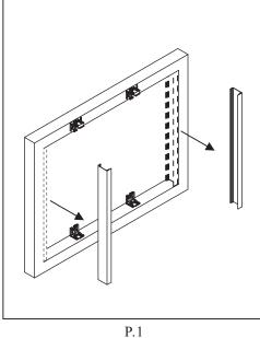
Install the window shade into the side rails.
