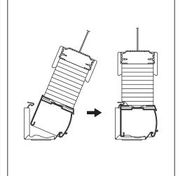
The bottom rail is installed into the head rail brackets at the lower end.
